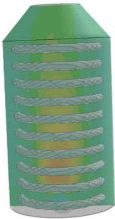
Figure 15: Process heater, temperature distribution
