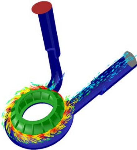
Figure 5a: Pump, velocity distribution
