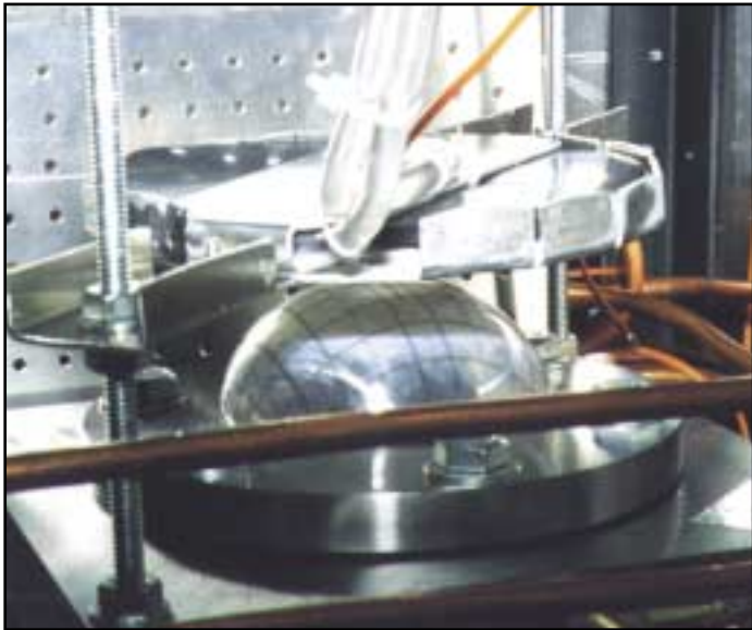
Biaxial inflation test rig for characterization of polymeric materials like PET, PS, PP, and PVC.
