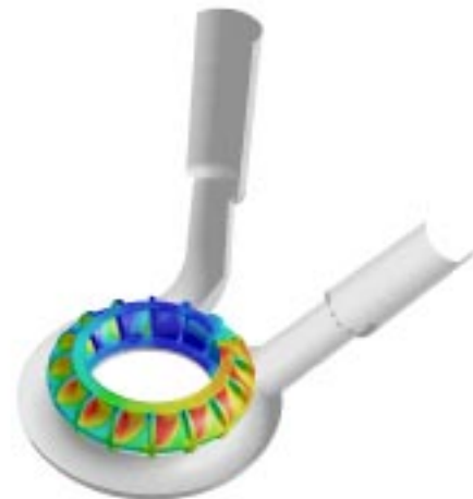
Figure 6 Pressure Contours on the Surface of the Poly-Pump Impeller
