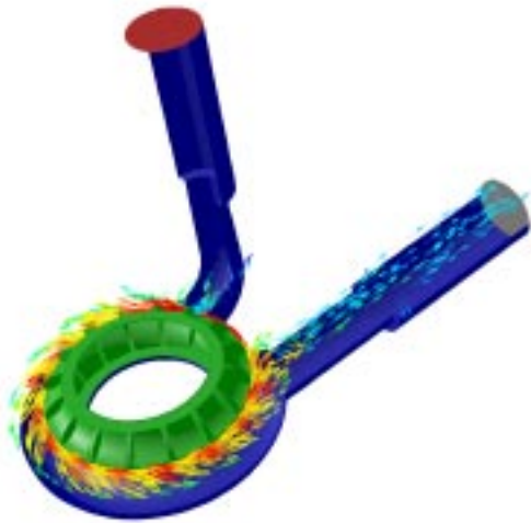
Figure 4 Velocity Vectors on the Center-Line Plane of the Poly-Pump Impeller
